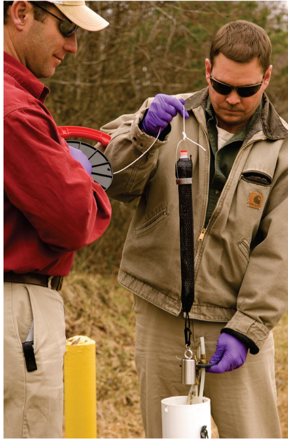
Fig. 4.36. Groundwater sampling at the Y-12 Complex. Technicians use a passive diffusion bag to sample for volatile organic compounds in groundwater.
